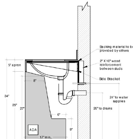
Note: Mount brackets to allow clearance for plumbing, optimal spacing between all brackets is 18" +/- 3".
