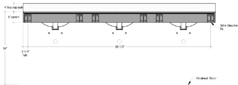
Note: Mount brackets to allow clearance for plumbing. Optimal spacing between all brackets is 18' +/- 3".
