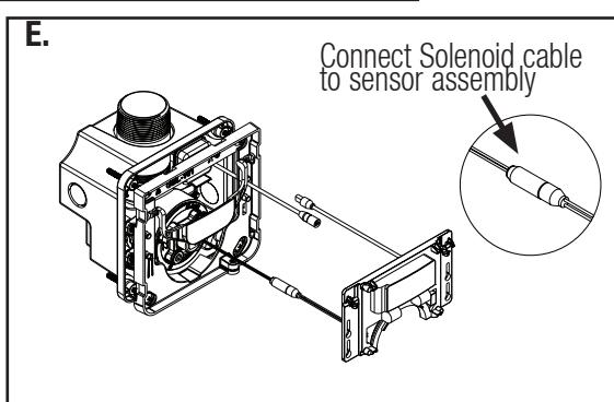
**The TruFlush Sensor assembly is designed to work with two options:**
