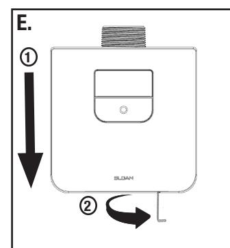
Flushometer is shipped with the flow control adjustment turned **OFF**.
